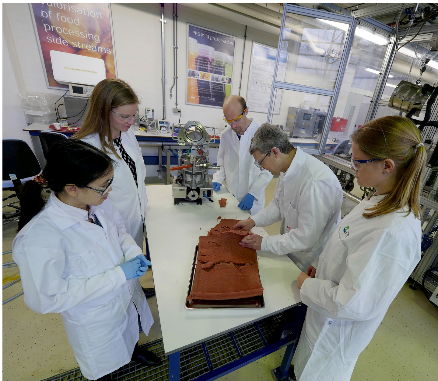
Scientists from Food Process Engineering (left; Nam Phuong Hua, Birgit Dekkers; right; Jacqueline Berghout, Atze Jan van der Goot, Jarno Gieteling) investigate a meat analogue, which is produced with an in-house developed equipment/ couette cell
